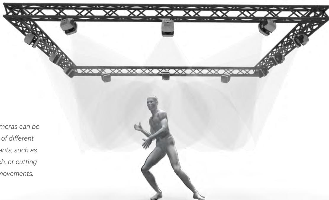
*In a 20' x 20' space, 12 cameras can be used to capture a variety of different full body athletic movements, such as a golf swing, baseball pitch, or cutting and jumping functional movements.*
