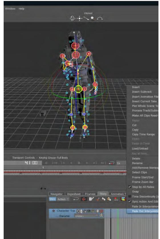
The Qualisys motion data is seamlessly streamed in MotionBuilder.
