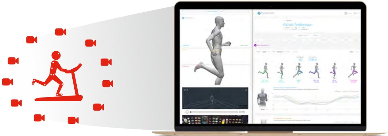
The system consists of 8 to 12 Qualisys motion capture cameras, depending on the lab's size and design. You get a 3D view from the front, back, and side, with all dimensions of the subject's movements, even rotations. Available analysis modules include Cycling, Running, Functional Assessment, Golf, and Baseball.
