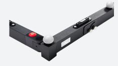
Our calibration frame includes height adjustment, spirit levels and alignment aids so it can be placed accurately on top of a force plate.
